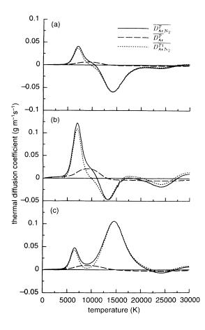
FIG. 6. Combined thermal diffusion coefficient, and its components, as a function of temperature for different mixtures of argon and nitrogen. (a) 10% argon, 90% nitrogen; (b) 50% argon, 50% nitrogen; (c) 90% argon, 10% nitrogen. Proportions are by weight.
